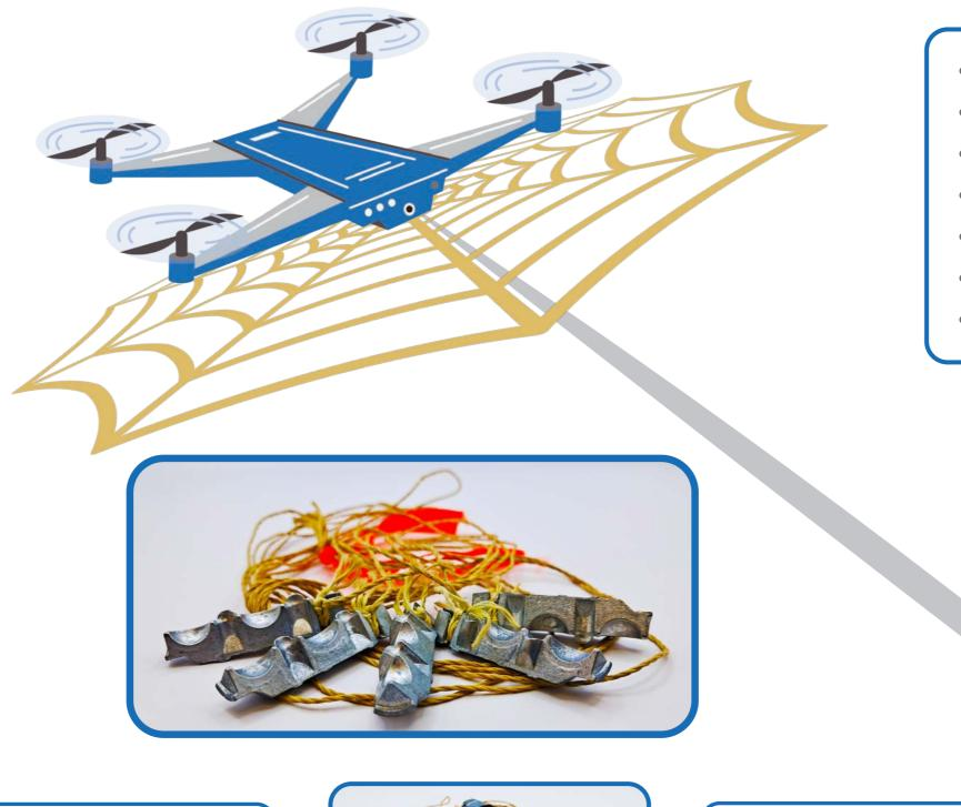
Upon deployment, the DB5 Kevlar web spans up to 1.5m (conditions dependent), with alloy weights designed to help maintain the web's full span.
