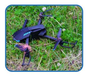
Upon interception, the DB5's Kevlar cords will wrap around the Drone's rotor blades, disabling the drone's flying capability, whilst preserving the drone for forensic investigation.
